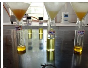
Fig J Filtration of acid digested material
