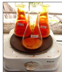
Fig I Acid digestion of dried powder
