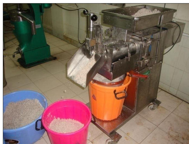
Fig 1 Coconut milk press (screw press)
