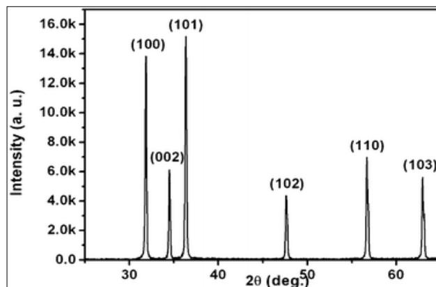
Fig 3 XRD pattern of ZnO nanoparticles
