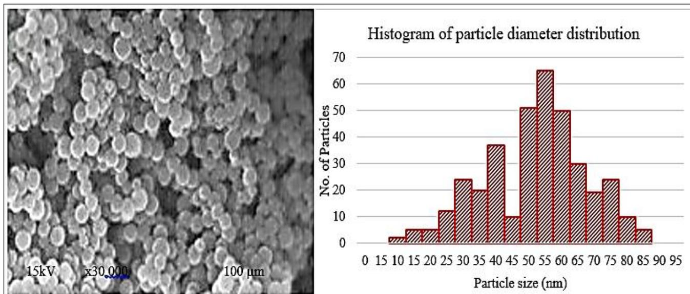
Fig 4 SEM images along with histogram of particle size diameter of ZnO nanoparticles
