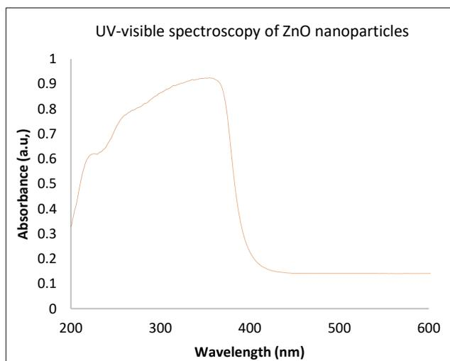
Fig 1 UV-Visible absorption spectrum for ZnO nanoparticles
