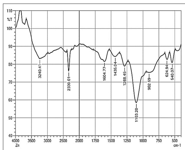
Fig 2 FTIR spectra of powdered ZnO nanoparticles
