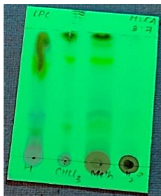
Fig 5 TLC Plates under UV light with mobile phase Hexane:Ethyl Acetate (3:7)
