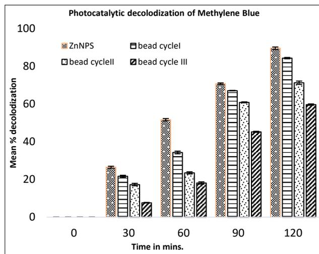
Fig 1b Photocatalytic decolorization of Methylene Blue (MB) by free and encapsulated ZnO nanoparticles
