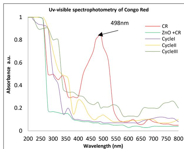
Fig 2a UV-Visible spectra of Congo Red, Congo Red +ZnO nanoparticles (CR+ZnO), encapsulated ZnO with repeated test for reusability testing Cycle I, Cycle II and Cycle III (The figure states the absorption spectra of Congo Red. Red color line depicts absorption spectra of CR. The absorption spectra for CR+ZnO, cycle I, cycle II and cycle III are shown by green, violet, yellow and blue lines respectively)
