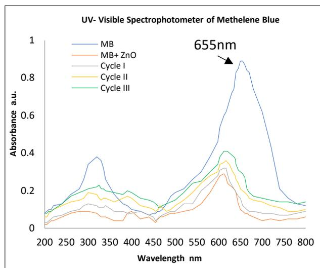
Fig 1a UV-Visible spectra of Methylene Blue, Methylene blue +ZnO nanoparticles (MB+ZnO), encapsulated ZnO with repeated test for reusability testing Cycle I, Cycle II and Cycle III (The figure represents the UV-visible spectra for Methylene Blue. The red line indicates identical absorption spectra for MB. The green, violet, yellow and blue lines indicate the absorption spectra for MB+ZnO, cycle I, cycle II and cycle III of MB decolorization)
