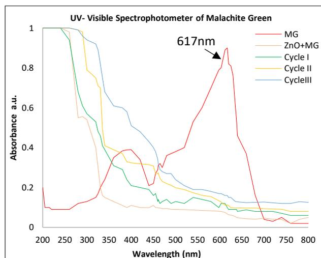
Fig 3a UV-Visible spectra of Malachite green (MG), Malachite green +ZnO nanoparticles (MG+ZnO), encapsulated ZnO with repeated test for reusability testing Cycle I, Cycle II and Cycle III (Above figure represents the trend of absorption spectra of MG, MG+ZnO, cycle I, cycle II and cycle III indicated by the lines in red, green, violet, yellow and blue color respectively)
