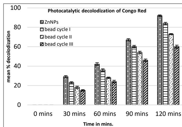
Fig 2b Photocatalytic decolorization of Congo red by free and encapsulated ZnO nanoparticles
