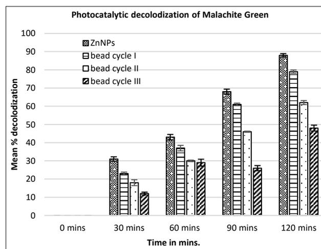
Fig 3b Photocatalytic decolorization of Malachite Green by free and encapsulated ZnO nanoparticles
