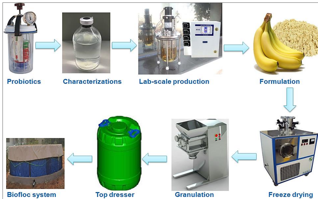
Fig 1 The process flow for the development of multi-strain shrimp probiotics on banana peel powder
