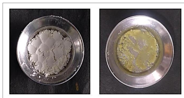
Fig 4 Hygroscopicity of the encapsulated powder
