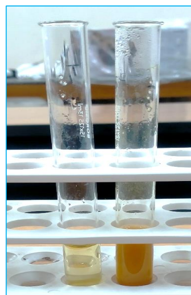
Fig 4 Benedict's test of Mosambi peel filtrate. Left test tube indicates only Mosambi peel filtrate and right test tube indicates Mosambi peel filtrate after reaction with Benedict's reagent. Appearance of red colour denotes presence of reducing sugar
