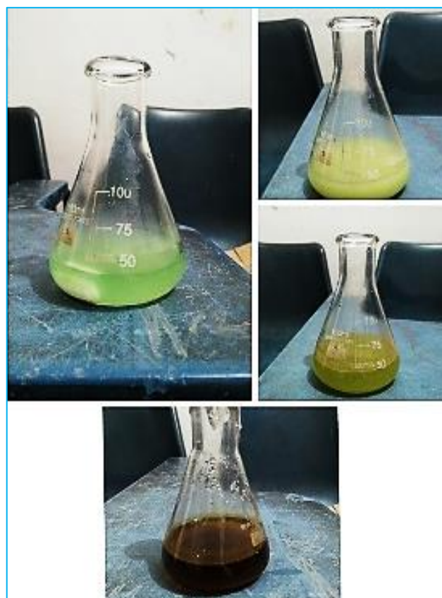
Fig 5 Confirmation by colour change reaction of CuNPs
