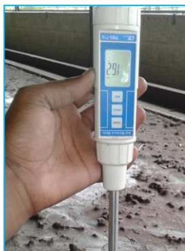
Fig 2 Soil moisture meter
