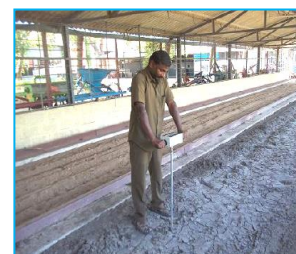
Fig 5b Soil cone index measurement
