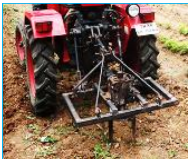
Fig 4 Single row vertical axis rotary tiller
