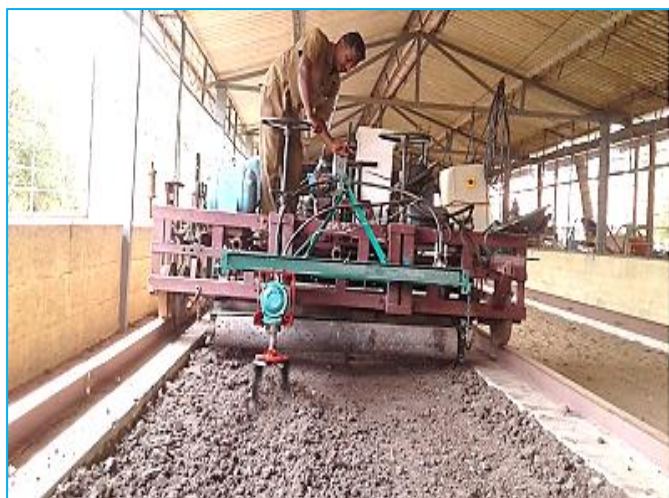
Fig 2 Experimental set up for measurement of torque for single row vertical axis rotary tiller
