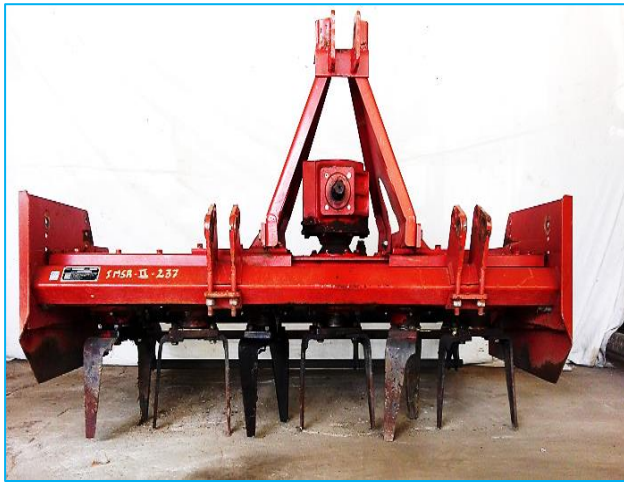
Fig 3 Ideal view of the modified six row vertical axis rotavator
