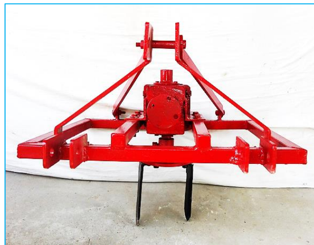
Fig 1b View of single row vertical axis rotavator
