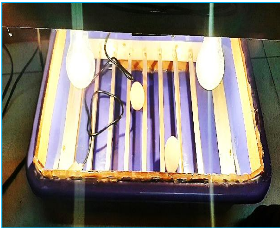
Fig 1 Schematic view of portable egg incubator
