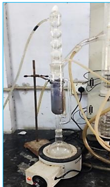
Fig 3 Steam distillation of mint
